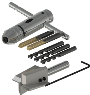
MH117-3B 1 in. (25.4 mm) diameter spot face and drill bit with 1/4-28 tap set
