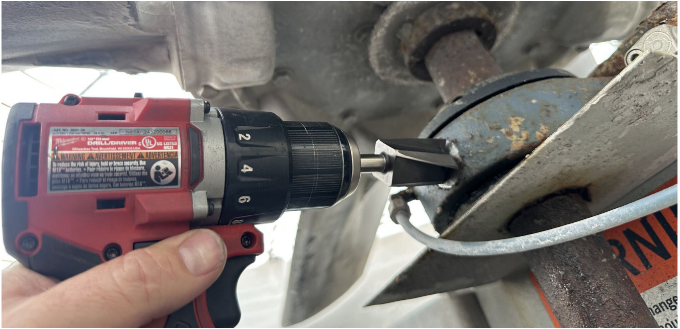
Fig. 1 Using a right-angle drill is key to creating a flat surface with the spot face tool
