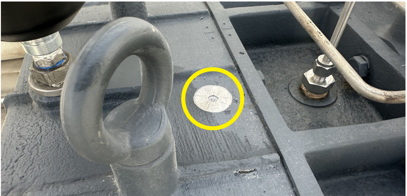
Fig. 2 Prepared surface for an adhesive mount
