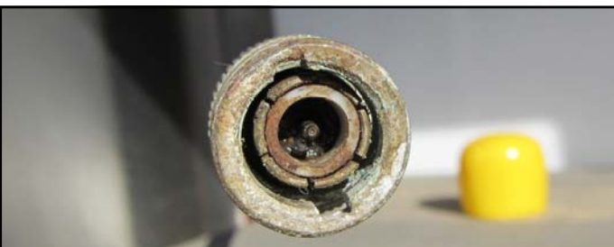
Figure 2— Close-up of male BNC exposed to severe weathering in a power plant. The yellow plastic cap did not provide adequate protection after less than 18 months.
