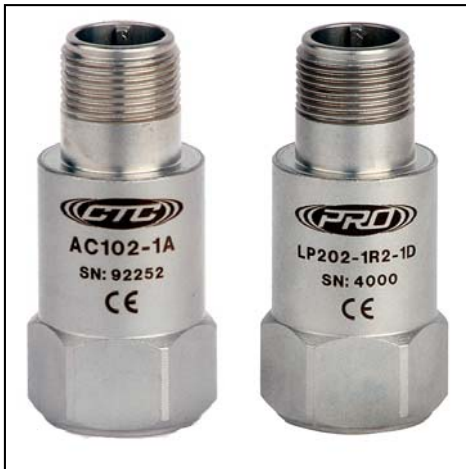
Figure 1—CTC’s dynamic AC102-1A accelerometer on the left and 4-20 mA output LP202-xxx-1D sensor on the right. The external form factor of both sensors is identical, as is the identical primary sensing element inside. The only difference lies in how the internal amplifier boards process the signal.
