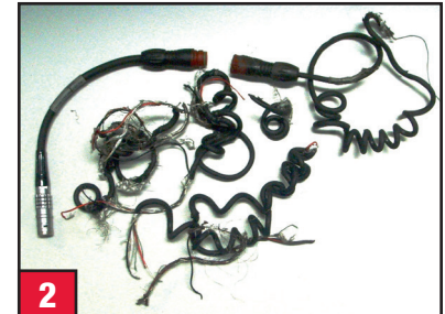
In this case, the safety connector saved the data collector and prevented a serious injury!
