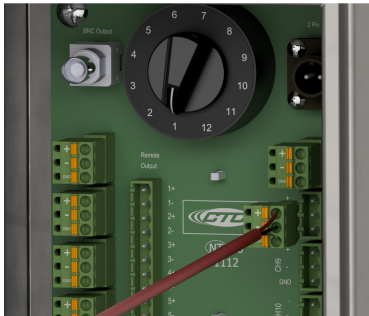
Figure 10. Connecting Cables to Switch Box
