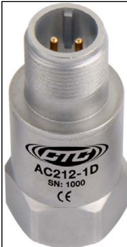
Figure 2— AC212-1D, 250 mV/g IEPE sensor for low frequency and slow speed applications requiring a higher g rating.
