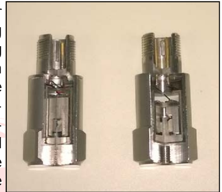
Figure 3— Side by side comparison of sensors. Note the smaller mass assembly in the sensor on the right and the larger mass in the sensor on the left.
