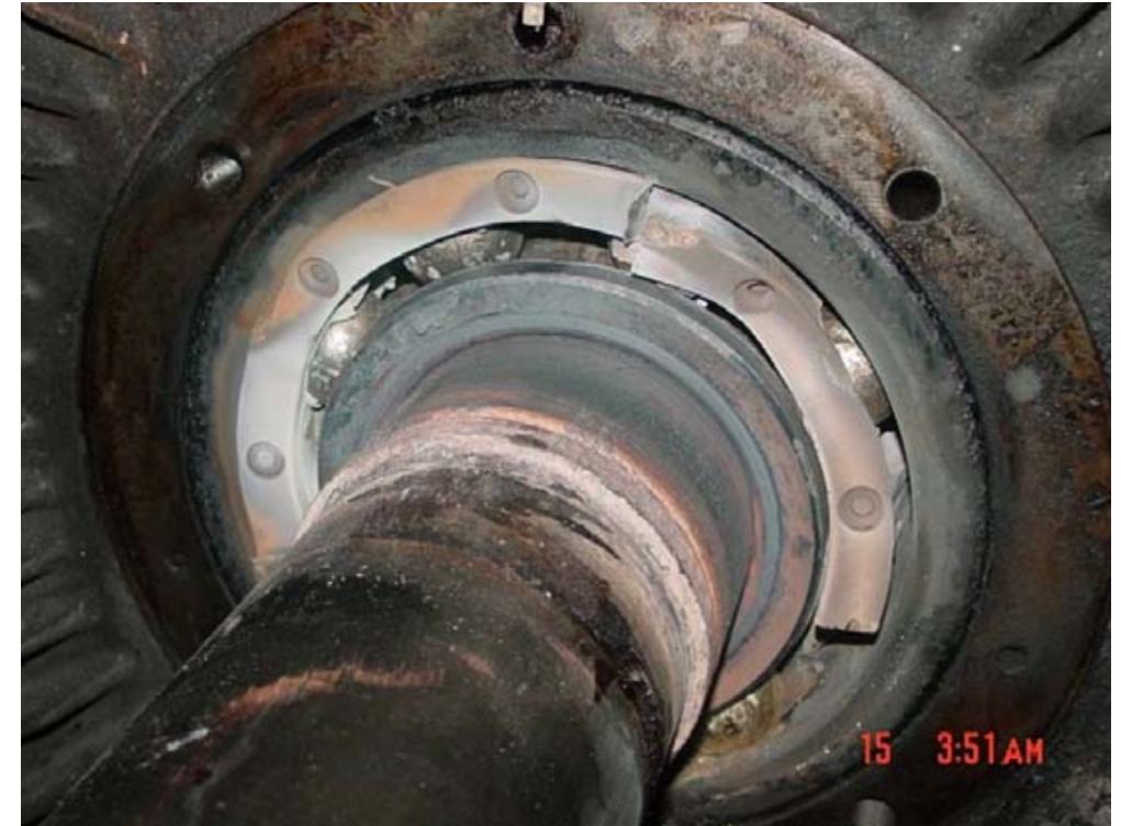
Failed Motor Bearing Don't Let This Happen To Your Machines !
