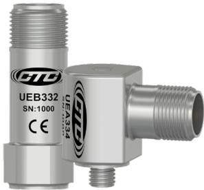
CTC's **UEB332** (top exit) and **UEA334** (side exit) sensor series combines a linear vibration output of 0.5 Hz - 23 kHz within a  $\pm 3$  dB tolerance. The resonant peak of this sensor is 42 kHz, which allows this one sensor to give a premium output in the vibration range and the ultrasound range.
