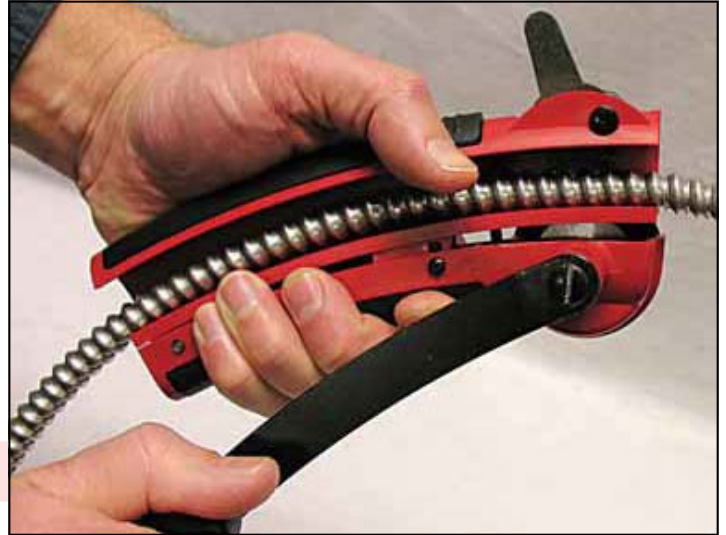
CB935-1A Armored cable cutter showing operation with larger cables. Exercise caution when using so as not to damage interior cable.
