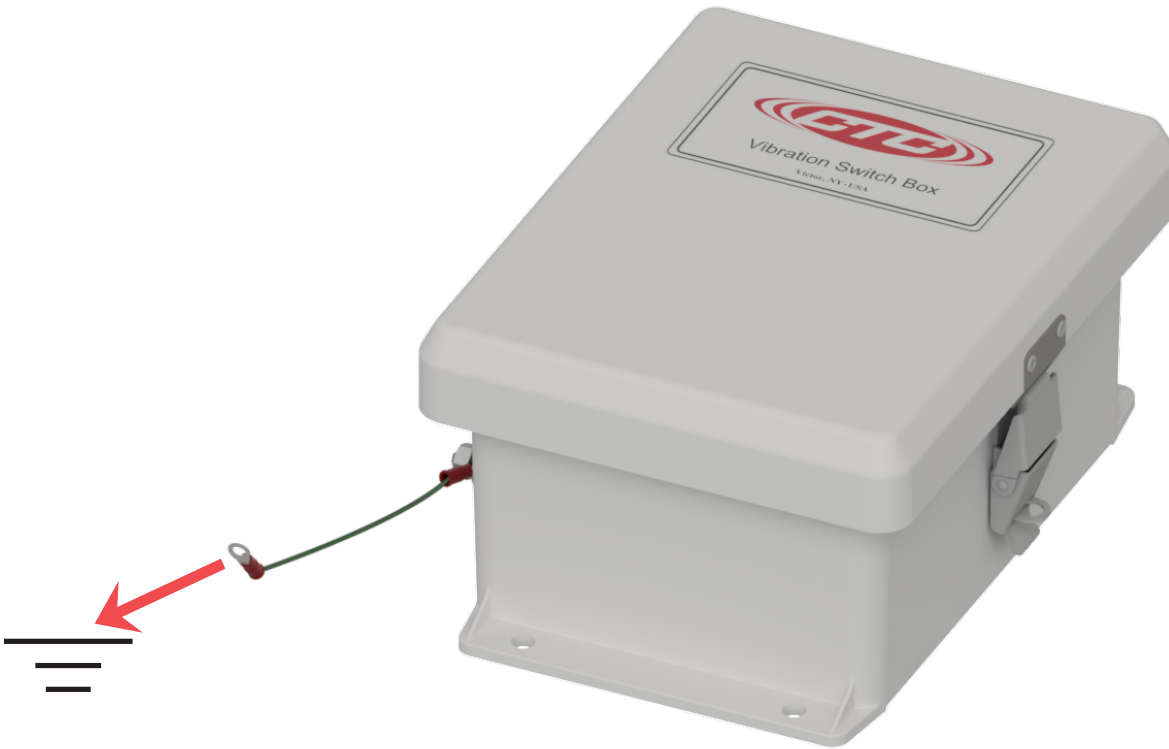
Figure 6. Ground Wire Placement
