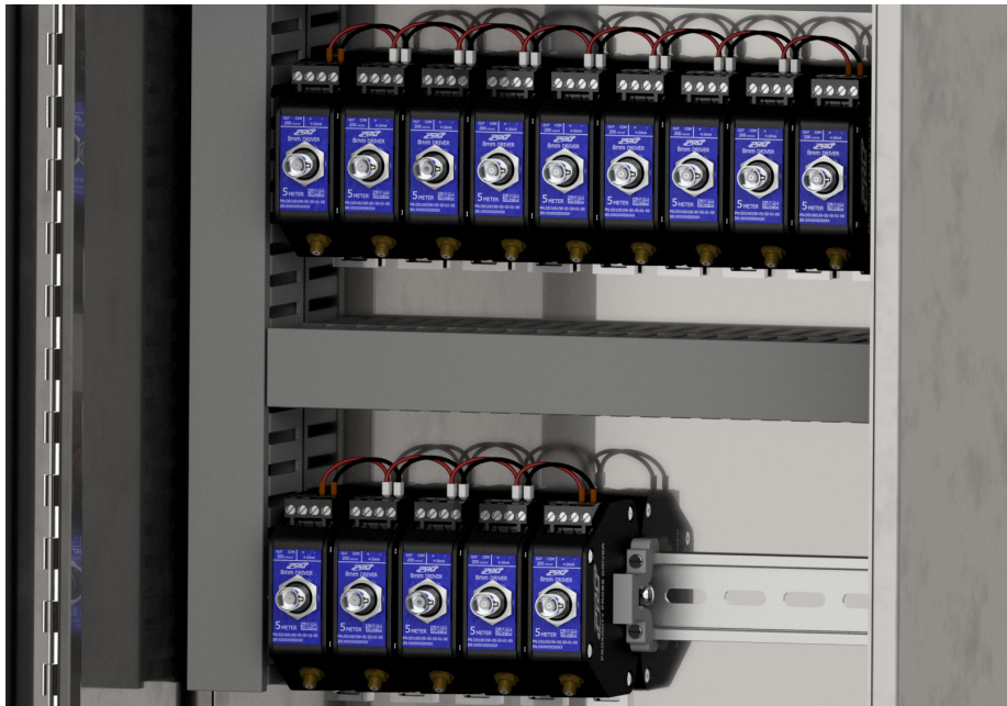
Figure 8. Power Routing for Probe Drivers
