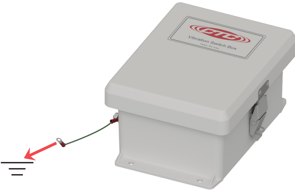
Figure 6. Ground Wire Placement
