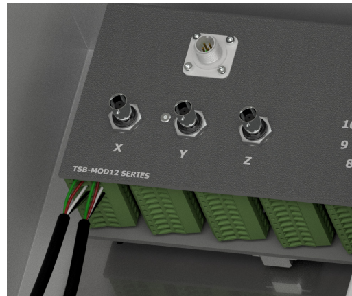
Figure 11. Connecting Cables to Modular Switch Box (TSB4001)
